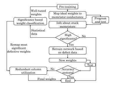
Figure 22. The overall flow of the technique of Liu et al. (figure adapted from [37]).
