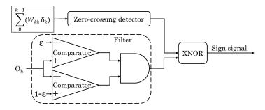
Figure 16. Sign computation circuit used by Li et al. (figure adapted from [35]).
