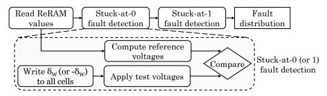
Figure 20. Checking for Stuck-at-0/1 fault (figure adapted from [20]).
