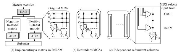
Figure 23. Mapping a matrix to MCA and two redundancy schemes (figure adapted from [21]).
