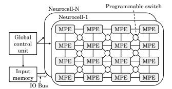
**Figure 35.** A reconfigurable core consisting of multiple neurocells, each composed of multiple MPEs (figure adapted from [15]).
