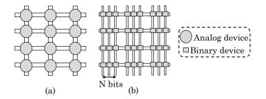
Figure 13. (a) Analog; and (b) binary-coded crossbar design (figure adapted from [41]).
