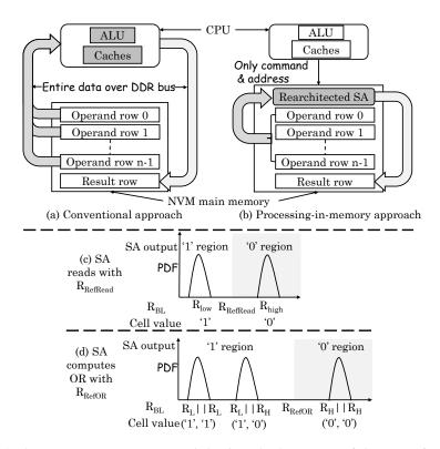
**Figure 24.** (a) The compute-centric approach leads to high amount of data transfer; (b) the PIM approach performs *N*-row bitwise operations in NVM in a single step; and (**c**,**d**) modifying reference resistance in SA to read the value and perform OR operation, respectively (figure adapted from [54]).
