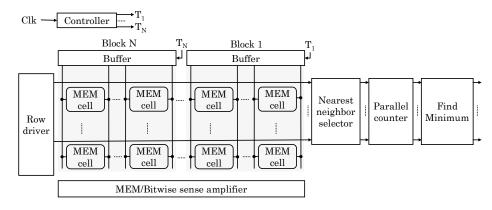
Figure 28. Circuit for searching nearest-neighbor (figure adapted from [59]).
