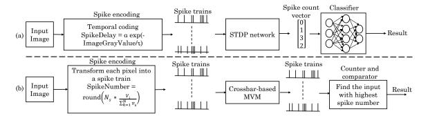
**Figure 36.** (a) Two-layer STDP based SNN (for unsupervised feature extraction) and three-layer ANN (for supervised classification); and (b) transferring ANN to SNN using neural sampling scheme (figure adapted from [44]).
