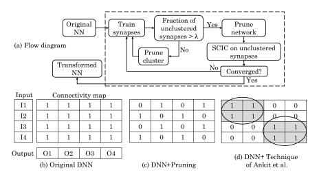
**Figure 10.** (a) Overall diagram of the technique of Ankit et al. [67], where  $\lambda$  is a threshold; and (b) an illustration of the impact of network pruning and the technique of Ankit et al. on a DNN connectivity matrix (here, 1/0 shows presence/absence of connection and not the actual weight) (figure adapted from [67]).
