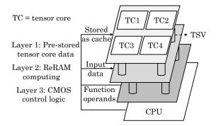
Figure 6. 3D CMOS-ReRAM accelerator for TNN (figure adapted from [19]).
