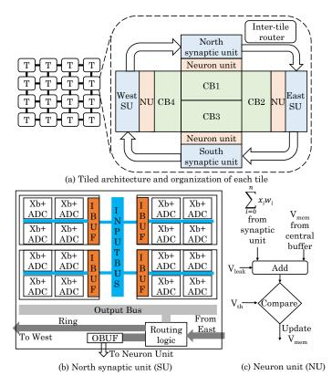
**Figure 37.** The technique of Narayanan et al. [45]: (**a**) pipeline diagram; (**b**) tiled architecture and organization of each tile; (**c**) north synaptic unit; and (**d**) neuron unit (S+A = shift and add)) (figure adapted from [45]).
