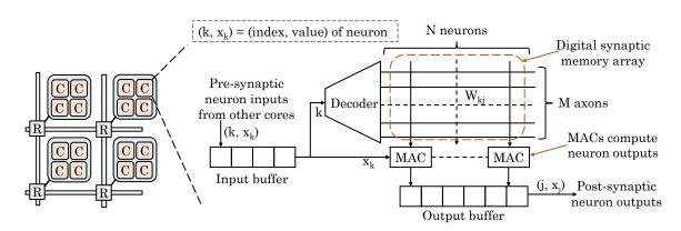
**Figure 5.** Digital neural core design (figure adapted from [57]). The analog core design [57] differs slightly from this design.
