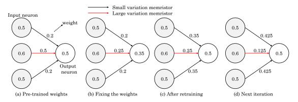
Figure 19. Illustration of change in weight during retraining of the network (figure adapted from [47]).
