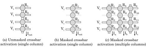
**Figure 12.** Masked and unmasked tree reduction in single and multiple columns (figure adapted from [41]).
