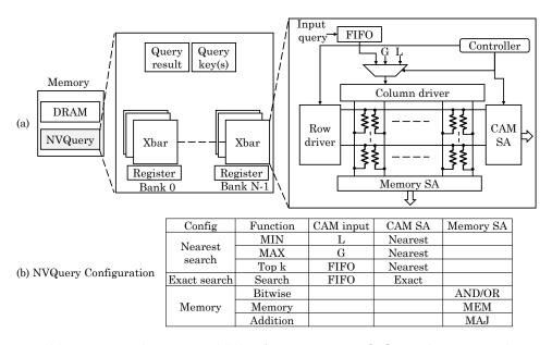
**Figure 29.** (a) NVQuery architecture; and (b) configuration settings [72]. G and L represent the greatest and lowest values, respectively. Empty cells in the table indicate that those inputs/settings are not applicable (figure adapted from [72]).
