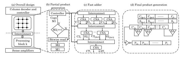
**Figure 26.** (a) Overall design proposed by Imani et al. [63], consisting of multiple data and processing blocks; (b) partial product generator; (c); fast adder tree composed of CSAs and configurable interconnects; and (d) final product generation for rippling the carry bits of tree structure (figure adapted from [63]).
