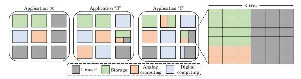
Figure 11. Field-programmable crossbar array architecture (figure adapted from [41]).
