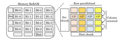
**Figure 33.** Streaming-apply execution architecture (src = source, dest = destination) (figure adapted from [53]).
